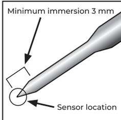
Apply the tip of the probe to the substance, medium or surface to be measured. The sensor is located at the tip of the probe, therefore the minimum depth insertion should be 3 mm. The probe tip is very sharp and therefore caution should be taken when using.
